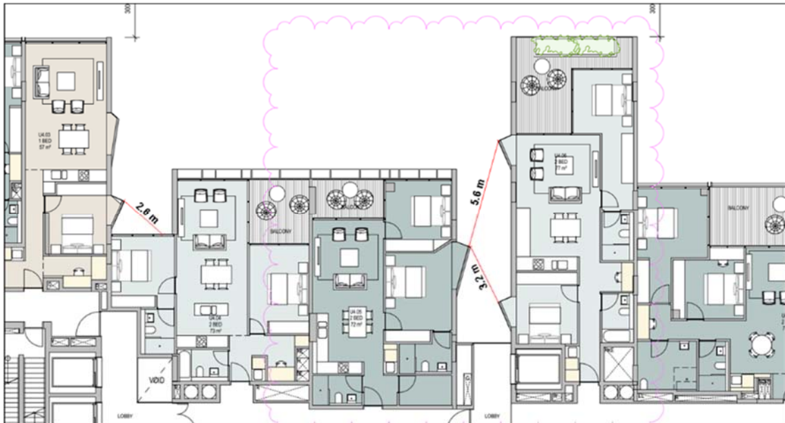
Figure 28: Example of separation between apartments in Building A.
