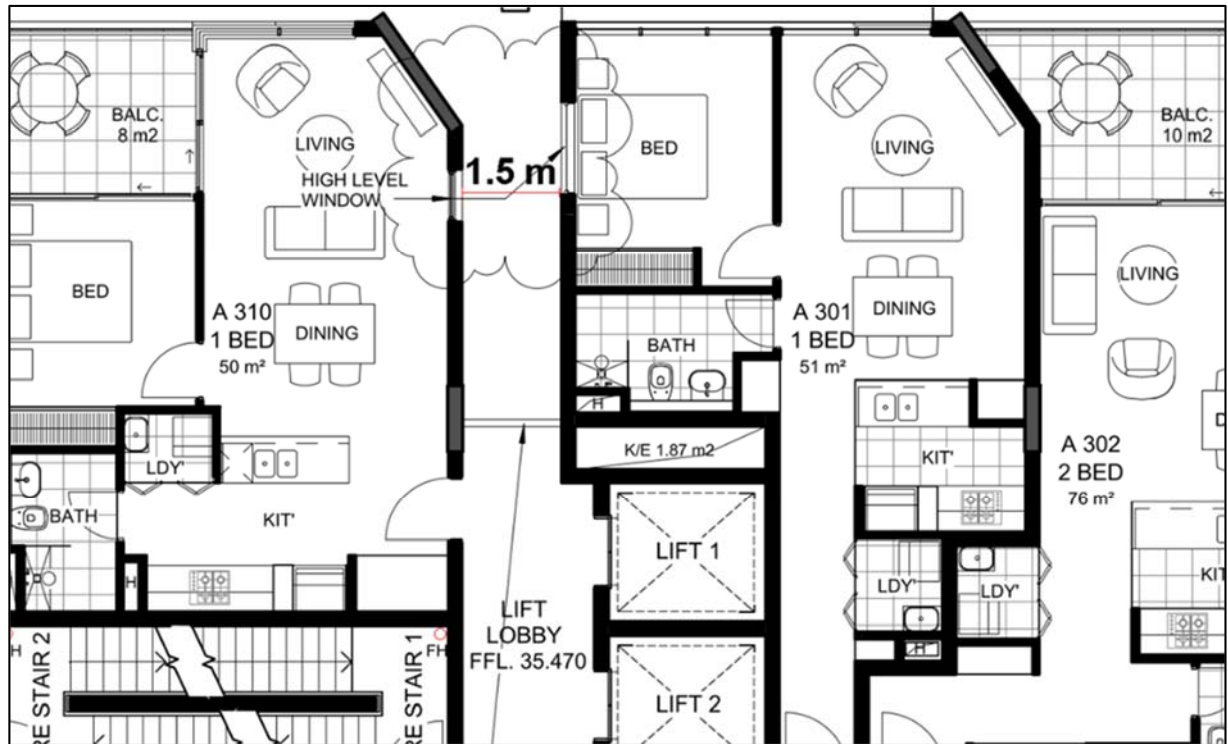
Figure 29: Example of windows within Building B that will require removal
